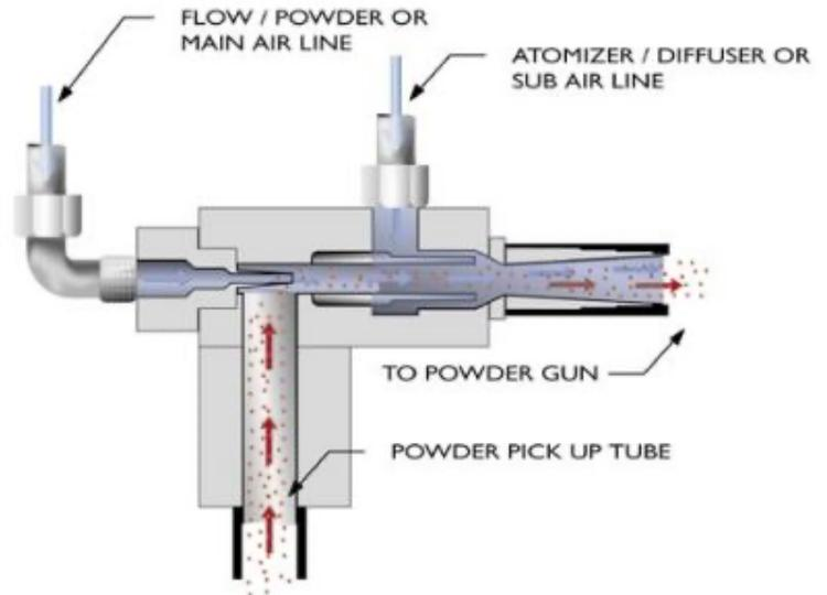
Fluidization pressure on a feed hopper can also noticeably affect the amount of powder being sprayed
