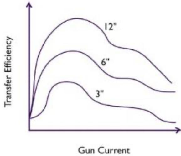
Transfer Efficiency vs. Gun to Part Distance
